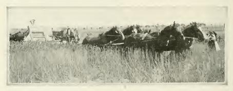
Harvesting wheat with the machine that cuts, thrashes and sacks the grain at one operation.
