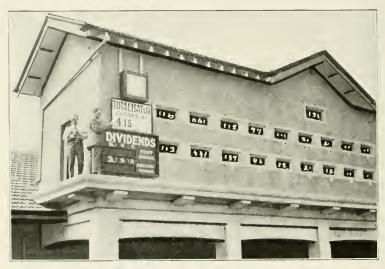
This is a photograph of the totalisator scoreboard. Under each slot is the number of the horse, and the figures in the windows indicate the amount "invested," or bet on the horse. The window at the top, near the roof, shows the total amount put up on the race, while at the left is a board showing the dividends which the winners pay. The "tote," as it is called, is the invention of a New Zealander.
