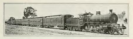
A modern passenger train in service between Melbourne and Albury on the Victorian railways. The passenger cars are built on American rather than European lines.
